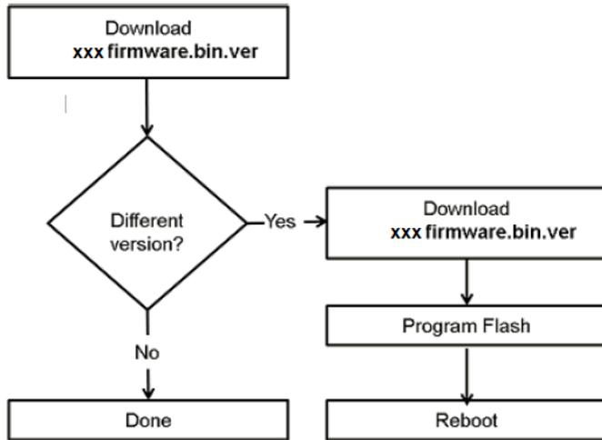
The firmware version specified in the ".ver" file is compared with the firmware version that is currently executed. To avoid problems with different firmware versions being executed and program flash, the Spectralink IP-DECT/DECT Server is rebooted immediately after the firmware is updated.
