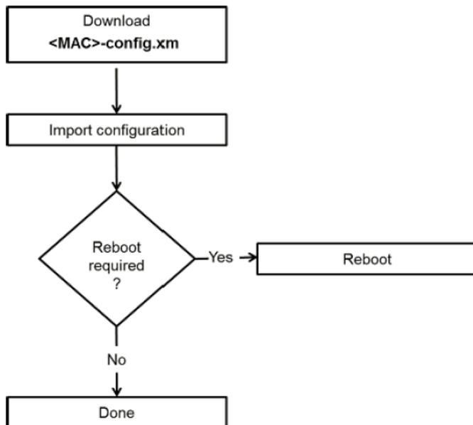
The XML configuration file is downloaded and imported into the Spectralink IP-DECT/DECT Server configuration by replacing the existing data. This guarantees that the data located on the provisioning server and on the Spectralink IP-DECT/DECT Server are identical.
